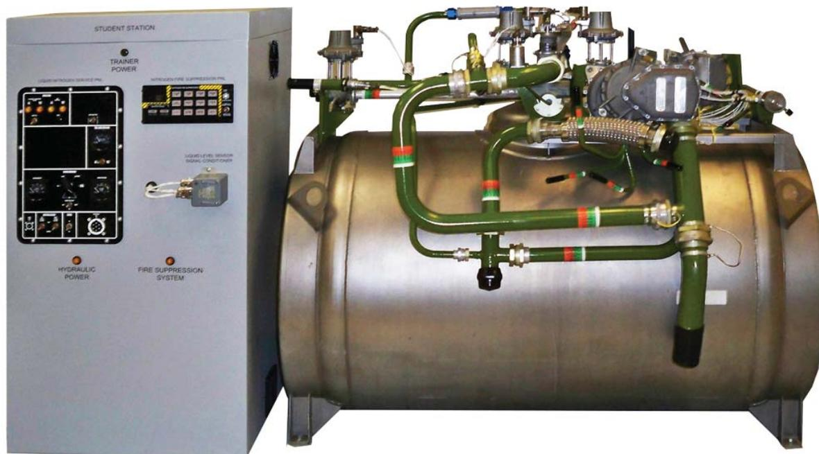
The trainer provides a full 360-degree view with walk-around access to all components. Instructors can teach hands on Remove and Replace procedures to a classroom of students in a fraction of the time it would take on an aircraft and without the potential for damage to otherwise operational flight-line equipment.
