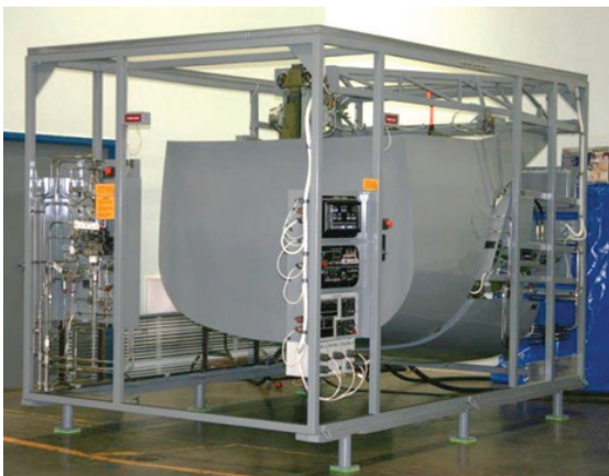
Trainer Forward Loading Panel (Panel 1) includes the Left Hand Forward Loadmaster Control Panel, Flight Station Control Panels, Associated Circuit Breaker Panels and the Air Delivery System.
